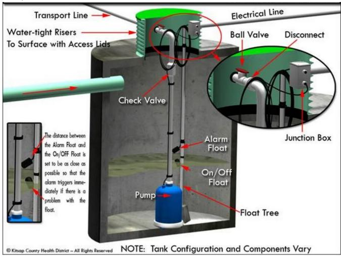
**NOTE:** If the drainfield is located below the pump tank an anti-siphon valve must be installed.
